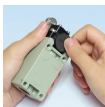
Loosen the cam holder with a coin or screw driver
